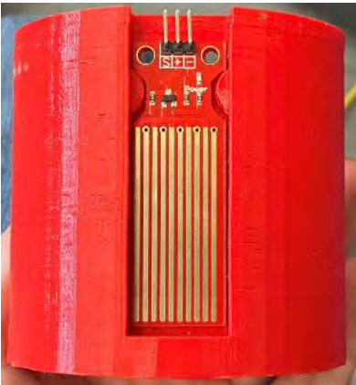
Brace leak sensor slot
