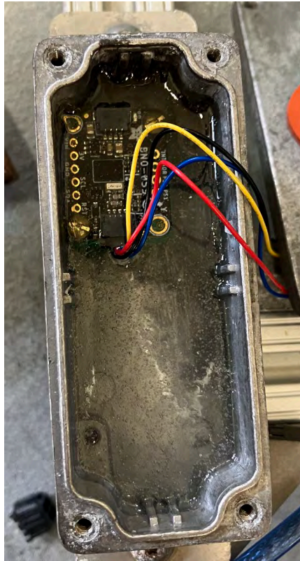
Replacement IMU unit set in resin
