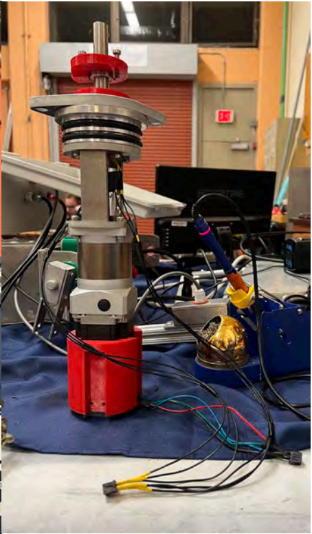
Replacement motor, fitted with a brace and connectors
