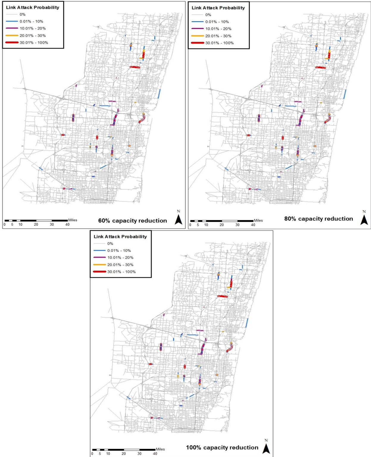
Figure 5. 18 Link's attack probability for 30 links per set under three different capacity reduction (60%, 80%, and 100%), Link attack selection: BC *
