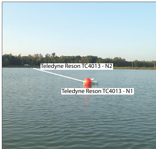
Figure 3. Underwater transducers are held by the red buoys and are deployed 322 ft apart.
