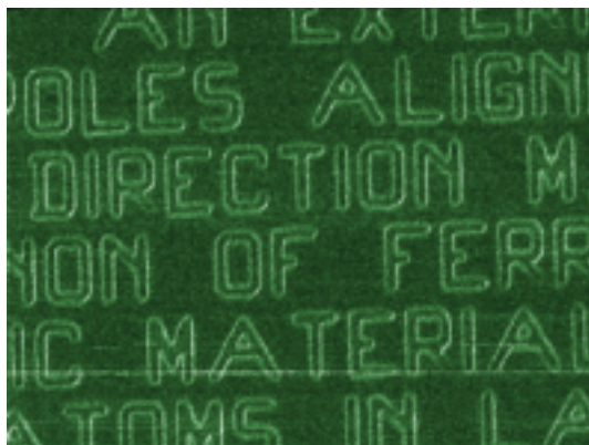
Figure 4 Nanoscale writing of a passage from the Encyclopaedia Britannica on a plastic slide or biochip, using a scanning electron microscope (used with permission, © 2004, Nanoscience Centre, Cambridge University, UK).
