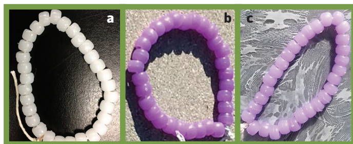
Figure 1 A sample UV bead bracelet (a) after no exposure to sunlight; (b) after full exposure to sunlight; and (c) after exposure to sunlight with a particular sunscreen
