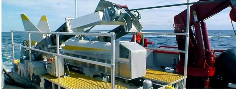
*Raytheon photo - Raytheon and FAU Harbor Branch perform developmental testing. The Littoral Combat Ship Variable Depth Sonar deployed and recovered at sea.*
